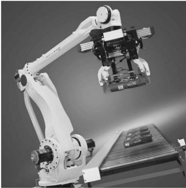
FIGURE 6.11 A FANUC M-410iB™ has 4 axes of motion. It is seen here performing bag palletizing
