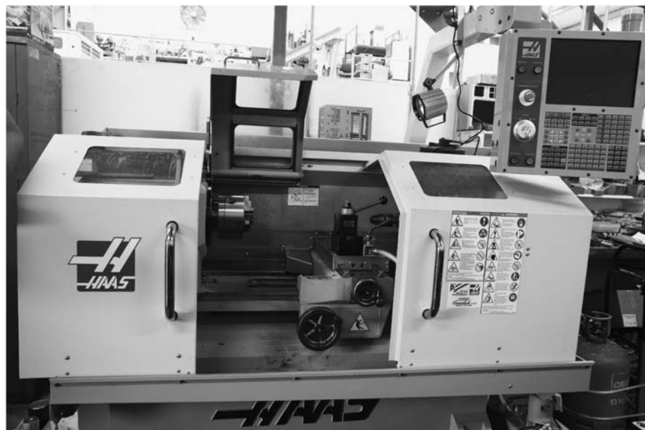
FIGURE 13.12 A lathe using digital numerical control
